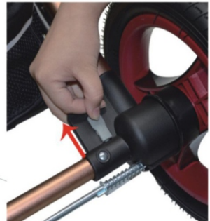
5. Slid Up the Piece to Disassemble Back Wheel
